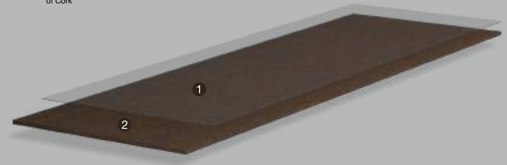
1 CORKGUARD® waterbased protection with CleanSurface technology 2 Expanded black agglomerated cork
